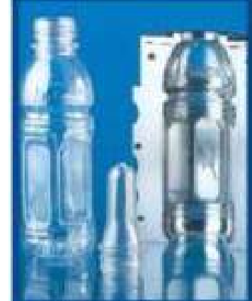
PET bottles, preforms, and moulding cavity
