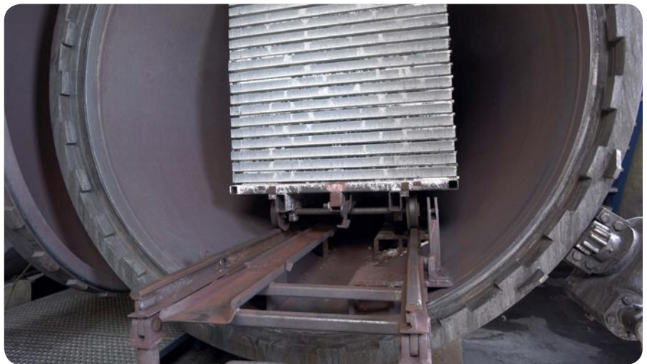
SKF extreme temperature bearings in the building material industry. Deep groove ball bearings in wheels of kiln trucks.
