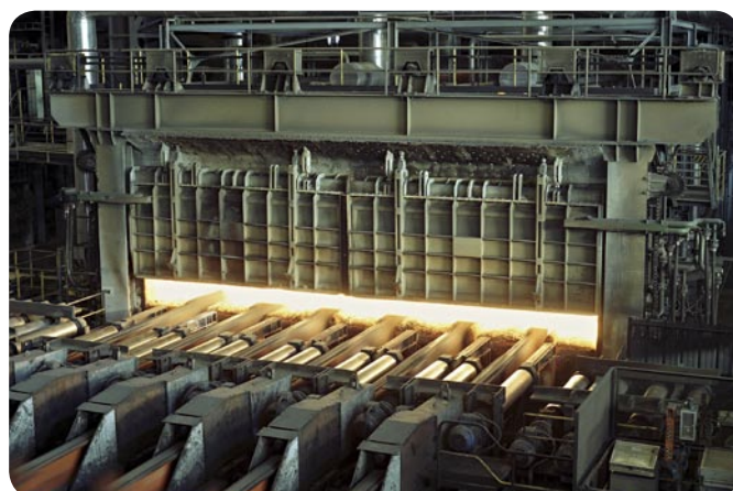
SKF DryLube bearings in the metal industry. Spherical roller bearings and spherical plain bearings in walking beam mechanism and in rollers outside of reheating furnaces.
