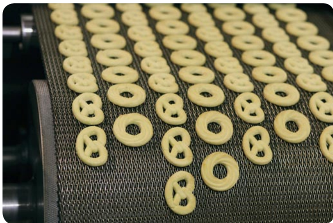
SKF DryLube bearings in the food and beverage industry. Spherical roller bearings in rollers of continuous biscuit ovens.
