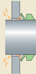
V-ring used as a grease valve
