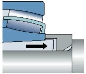
In addition, it must be possible to mount a suitable stop against which the hydraulic nut's piston can rest.
