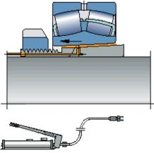
Connect the oil injection pump to the sleeve connection.
