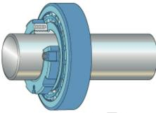
If the locking clip does not lign up with the slit in the adapter sleeve, a new locking clip has to be made, for instance according to the figure. Do not loosen the nut from the determined position.
