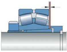
Push the bearing further up with the hydraulic nut but not more than it is still possible to remove the shims. Remove the shims and drive the bearing up until it contacts the spacer sleeve.
