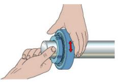
If the bearing is to be oil lubricated take care that the right quantity of the right oil is used.
