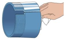
Lightly oil the bore of the bearing with a thin mineral oil.
