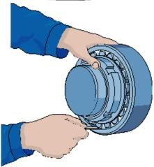
Before measuring, the bearing should be rotated a few times to ensure that the rollers have assumed their correct position.
