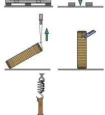
Use lifting equipment to facilitate the handling of the bearing. Spring suspension can simplify bearing positioning.
